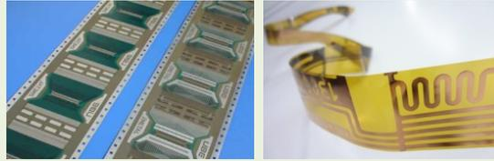
“UPILEX®-SGA” is a polyimide film having improved adhesion properties created by a special process to both sides of the “UPILEX®-S”. It is suitable for sputtering or plating processes because of high surface adhesion. It offers a flexible base for high-performance electronic circuits. In addition, it can also be used as an adhesive tape base material for LOC packaging.
