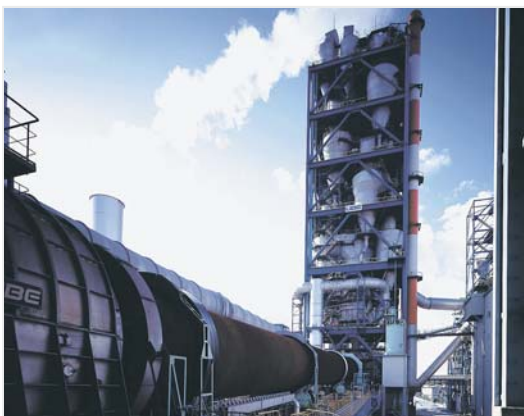
The new suspension preheater kiln at the Ube Cement Factory
