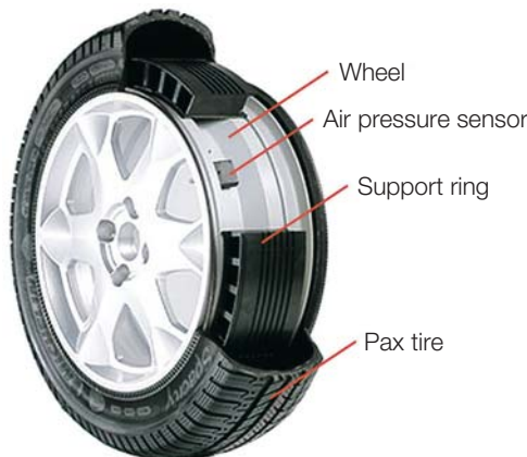
A look inside the run-flat tire system (PAX system)
