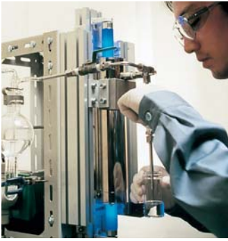
Dioxin decomposition experiment using fibrous photocatalyst
